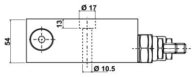
Maximum pressure 280 bar 4060 psi Pressure range 70-250 bar 1015 - 3625 psi Maximum rated flow 100 lpm Pilot ratio 4.25:1
