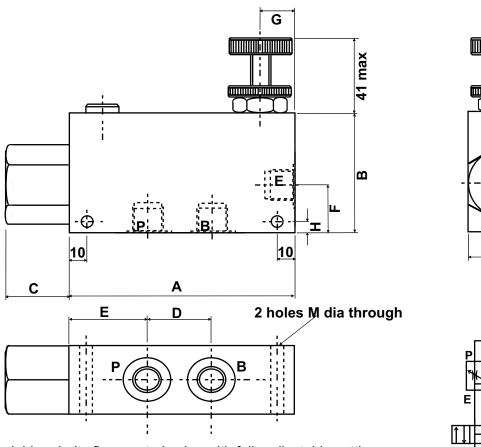
Variable priority flow control valve with fully adjustable setting. These valves split a single input flow into a priority regulated flow and a by-pass flow which can be used in a second circuit or to tank. Constant priority flow is maintained regardless of any fluctuations of input flow or pressure.
